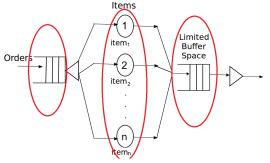
Challenge: Determine optimal delay for each item in order so that item for the same order arrive in output buffer at approximately the same time.
